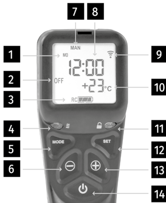
Fig. 11. Remote control type FB 868D (TESC) 1 - Day of the week, 2 - Heater status, 3 - Battery indicator, 4 - Light sensor, 5 - Mode selection, 6 - Decreases the flame button, 7 - Current mode, 8 - Hours and minutes, 9 - Connection with the heater indicator, 10 - Ambient temperature, 11 - Remote control lock indicator, 12 - Entering settings, 13 - Increase the flame button, 14 - Turn on / off
