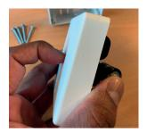
2 Push and hold the button on the front of the room temperature sensor for 4 to 5 seconds until the sensor starts flashing sequences of green and red light.
