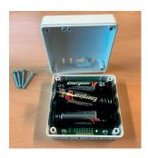
Make sure there is no power connected to HWAM® Smart-Stove™. Remove the lid of the room temperature sensor and insert 3 AA batteries.
