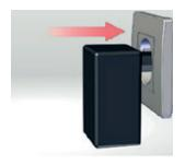
3 Plug in the stove's power supply within two minutes. The room temperature sensor will keep flashing green and red lights. Then the green light will flash 5 times, and when the light goes out, the sensor has been correctly paired with the wood-burning stove. The distance between the room temperature sensor and the stove may be up to 4 to 5 meters.
